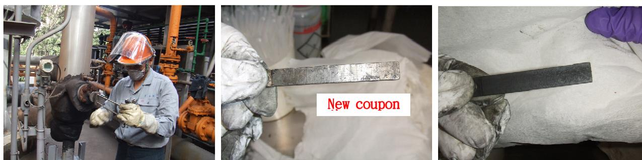
**Fig.12.** Photographs of the anti-corrosion film formed on the surface of a coupon.
